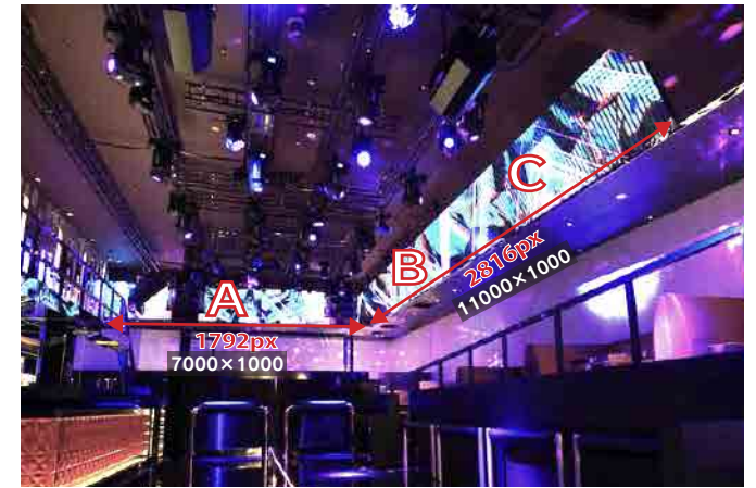
LED VISION (ピクセルピッチ:3.9mm)
